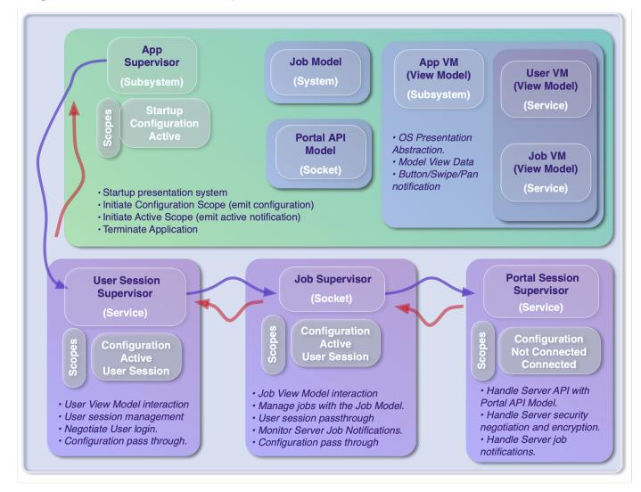
Explaining the operation of this design, the **App Supervisor** element manages the whole system and so is the causal initiator of system. It has a number of operational states (termed **Scopes**) for:
